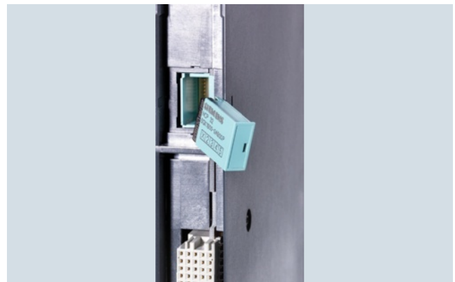
Plugging the C-PLUG into the rear of the CP 443-1 Advanced
